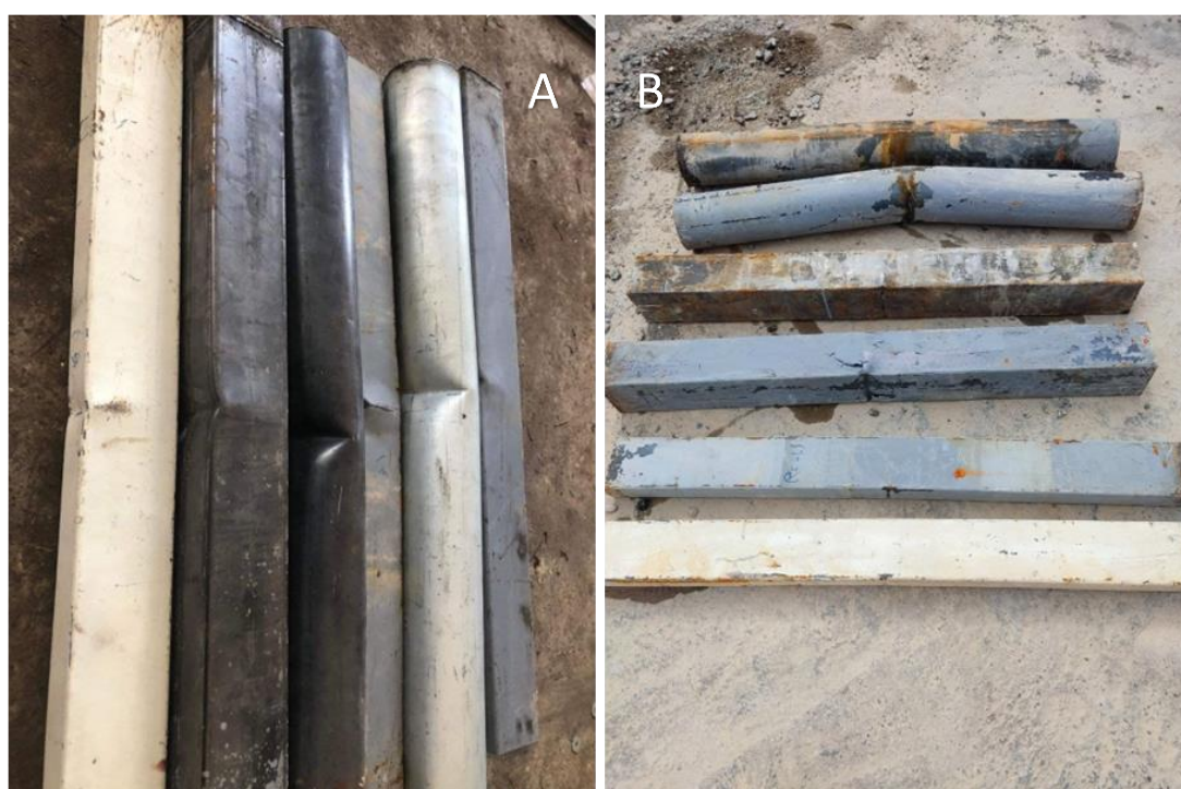
Figure 6. Group of steel tube failure mode, A) Hollow steel tube, B) CFST beams
