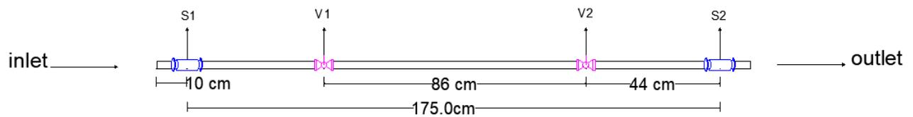
**Figure 2.** Equivalent pipeline system
