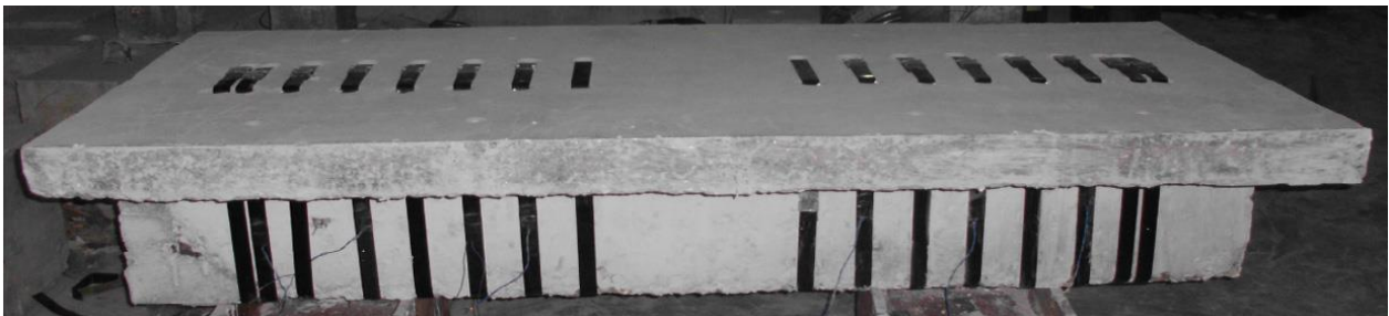
Figure 6. Slabs were drilled to create paths for the metal straps [21].
