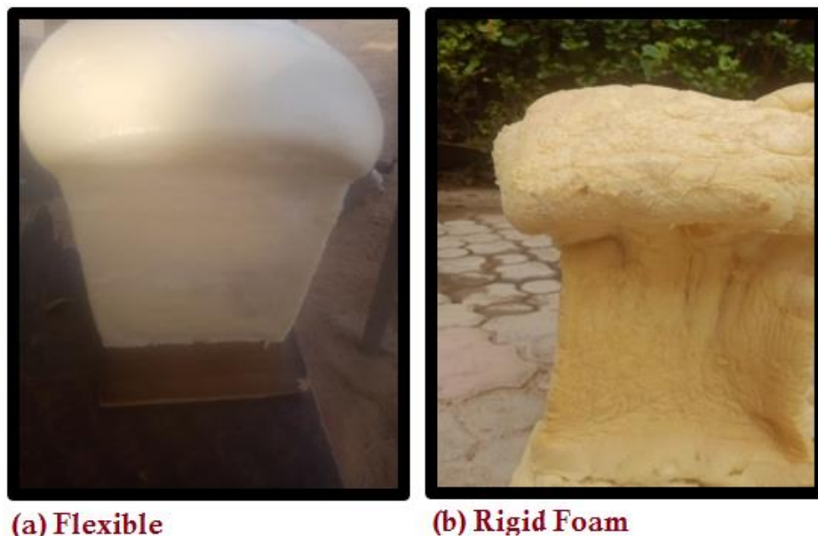
Figure 1. (a) Flexible Formulation A and (b) Rigid Formulation B Foam
