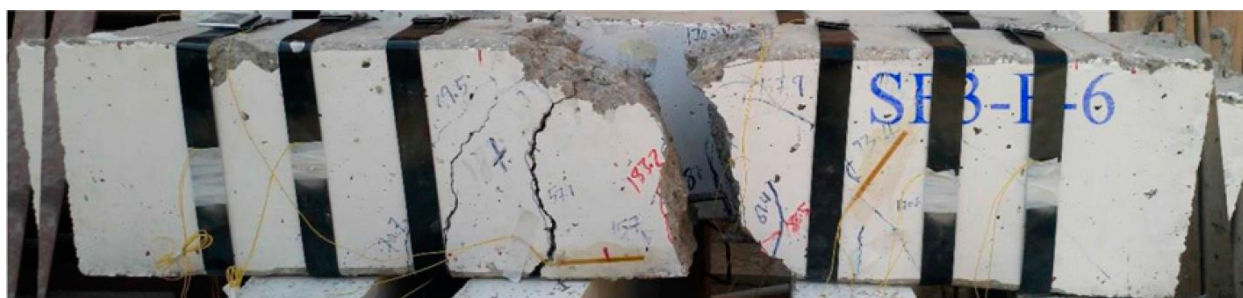
Figure 15. Changing behavior of the beam failed in shear to bending [8]
