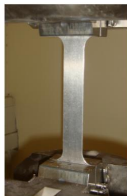
(b) Coupon specimen mounted in UTM
