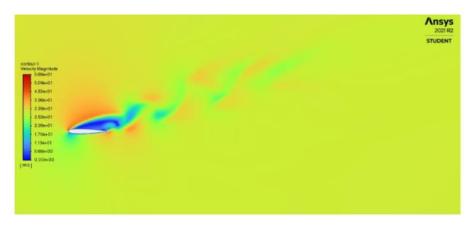
Figure 13. Velocity contour at 20 degrees AoA
