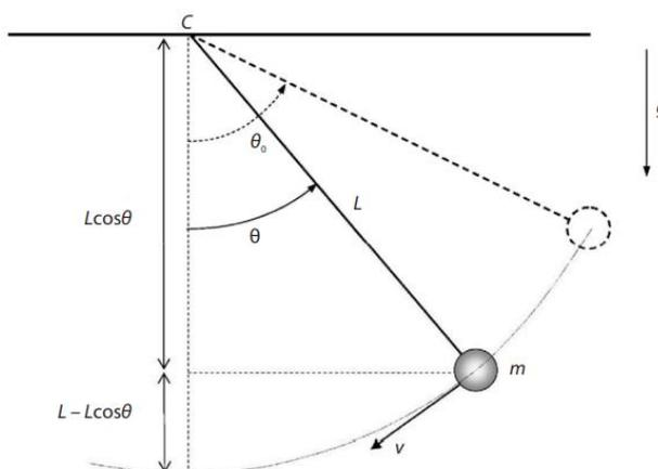
Figure 1. Scheme of a simple pendulum motion [22]
