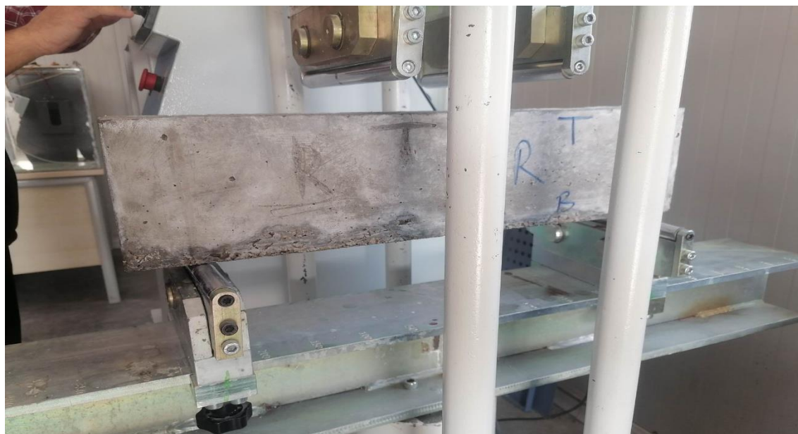
Figure 2. Four-point bending test setup
