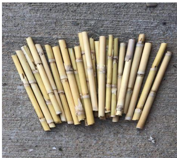
Figure 2. Bamboo cut to be used as vertical legs
