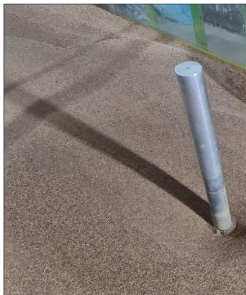
Figure 4. Cylindrical aluminum pier model.
