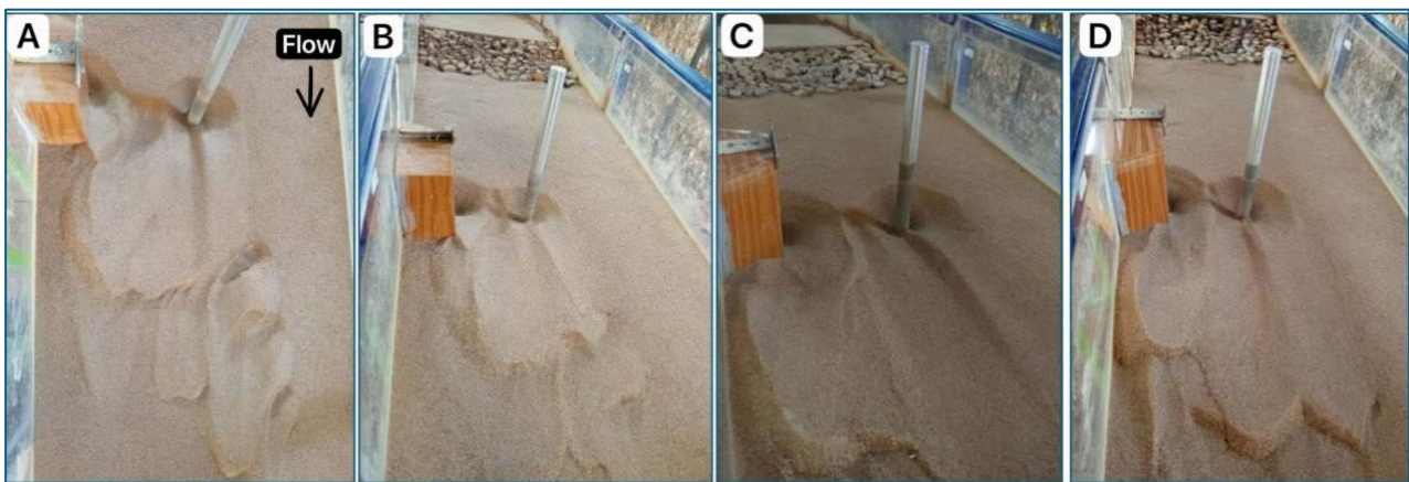
Figure 11. The scour hole development at the same conditions, y=9 cm and v/v_c=0.7 , for the trapezoidal model (A, at x=22.5 and B, at x=17.5 cm) and the wing-wall model (C, at x=22.5 and D, at x=17.5 cm)
