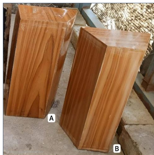
Figure 3. Wooden abutment models (A) trapezoidal, and (B) wing-wall.
