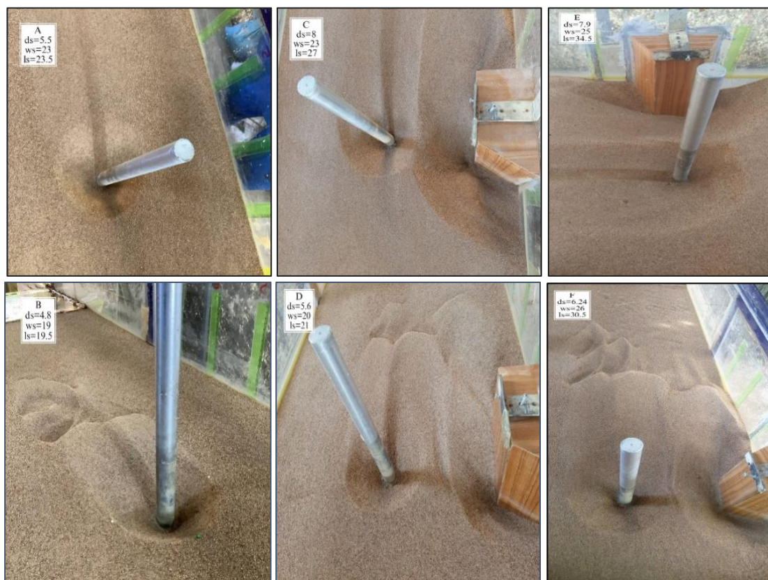
Figure 10. The effect of increased flow depth with constant distance between pier and abutment x=22.5 cm, and constant discharge on scour hole development around the pier. (A-C-E) RUN 7 at y=9 cm, and (B-D-F) RUN 9 at y=11 cm. All scour hole dimensions in cm.
