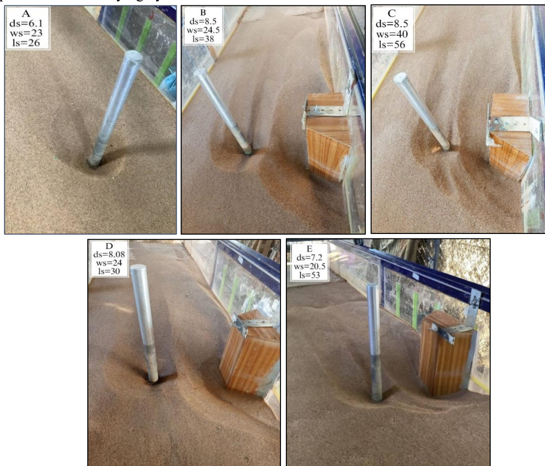
Figure 8. The development of scour hole according to effect of high flow intensity v/v_c=0.9 and y=11 cm at (A) pier only, (B) interface between trapezoidal shape and pier at x=22.5 cm (C) Trapezoidal at x=17.5 cm (D) wing-wall at x=22.5 cm (E) wing-wall at x=17.5 cm. All scour hole dimensions in cm.
