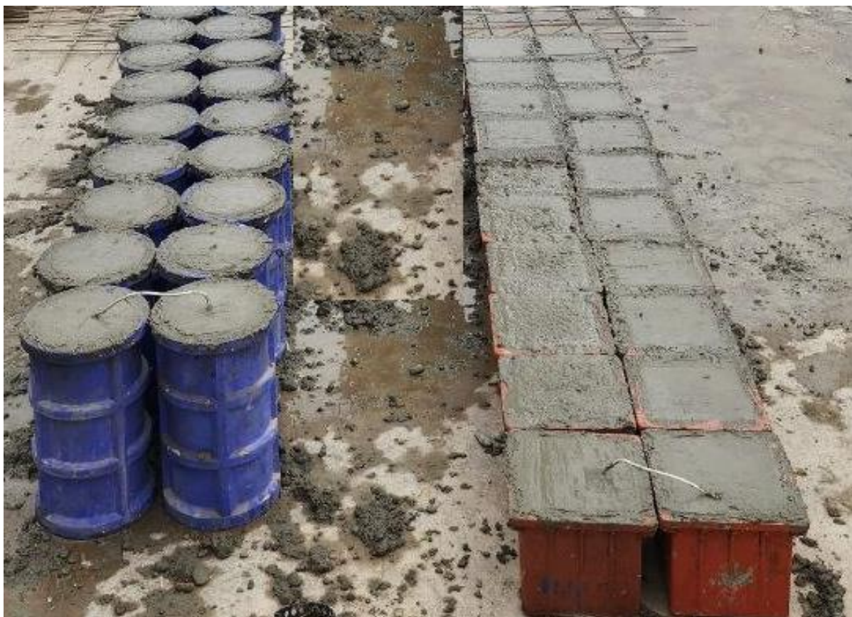
Figure 4. Cylinder and cube specimens used for compressive strength testing, showing their size and shape
